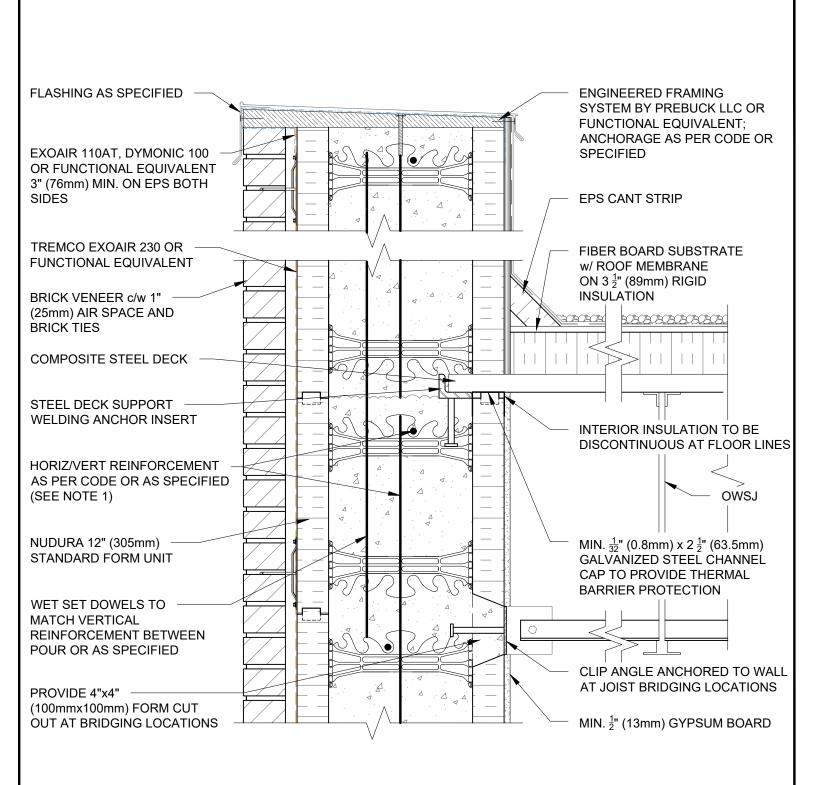
1) FOR OPTIMAL REINFORCEMENT PLACEMENT IN THE NUDURA FORM, SPACING OF HORIZONTAL REINFORCEMENT TO BE SPECIFIED AT 18" (457mm) O.C. AND VERTICAL REINFORCEMENT TO BE SPECIFIED AT MULTIPLES OF 8" (203mm) O.C. REFER TO NUDURA REINFORCEMENT PLACEMENT DETAILS.
